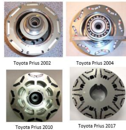
Figure. 6. Design trend in rotor of Toyota Prius over the years from 2002 to 2017.
