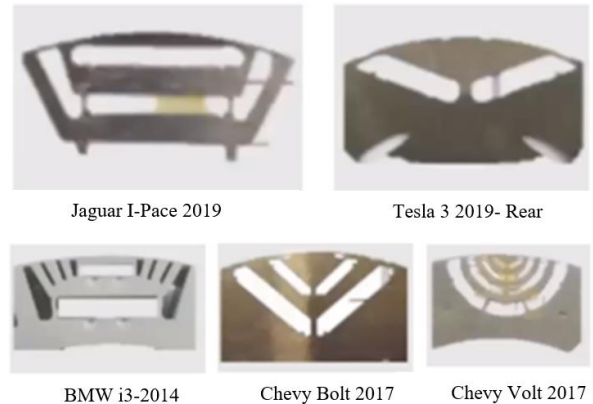
Figure. 7. Design trend in air barrier type rotors of PM-SyRM by different manufacturers.
